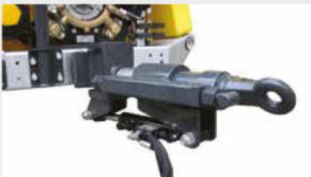
Steering drawbar with towing eye and hydraulic locking.
