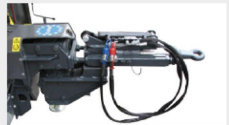
Steering drawbar with gear transmission and hydraulic locking.
